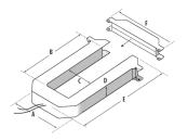
800 - 2400 Amp A= 4.9" (124 mm) B = 5.5" (140 mm) C = 2.5" (62 mm) D = 1.1" (29 mm) E = 8.1" (207 mm) F = 5.9" (150 mm)
