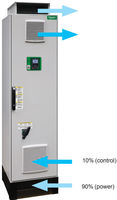
UL Type 12 cooling system with separate air flows
